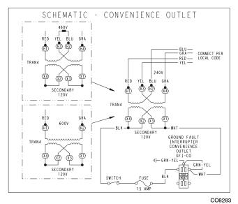
Fig. 15 - Powered Convenience Outlet Wiring
